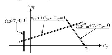
Figure 1. Linearised "cap model" for unreinforced masonry wall ( $f_t$ : mortar adhesion, c: mortar shear strength,  $f'_m$ : block compression strength)
